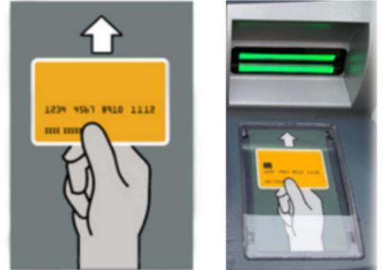
For increased security, our ATM card readers now require that the ATM card be inserted long-edge, instead of the traditional short-edge orientation, making it difficult to capture the card's information with current skimming technology.
